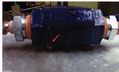
Figure 3A: Failure mode of Sample# 13-06-C0161-2, Body fractured at 6,613 psi.
